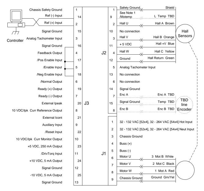
Note 1: Motor's thermal switch, if equipped, is wired so motor overtemperature causes Amplifier shutdown. If motor has no switch, connect a jumper between /Motemp and Ground.
